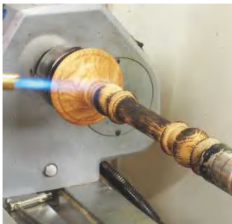
▲ Pic.31 Using a gas torch, lightly burn the surface – as the timber is wet you are less likely to remove all the shape. The burning will remove some of the softer growth from the timber and soften detail, mimicking the ageing process
